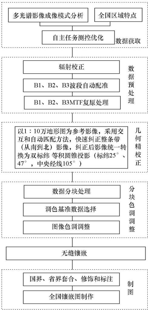
图 2 北京 1号小卫星全国镶嵌图制作技术流程图 Fig.2 The workflow map of China's digital mosaic map based on the multispectral images of Beijing-1 Microsatellite
