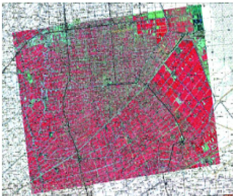
图 8 几何纠正效果示意(与 1:10 万地形图套合比较) Fig.8 The geometric corrected map of test site (overlayed with 1:100, 000 relief map)
