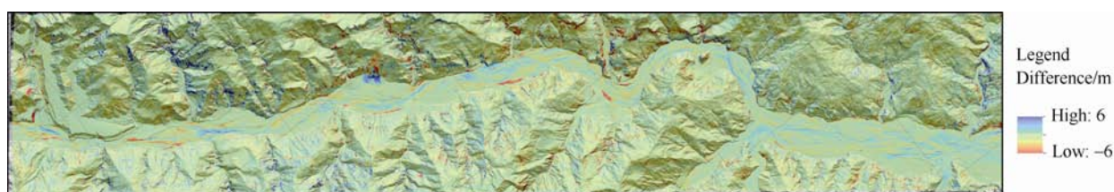
Fig. 5 Overlay of elevation difference values before and after the typhoon season on terrain shadow map for after the typhoon season
