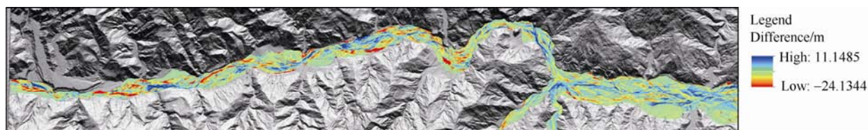
Fig. 6 River elevation difference values before and after the typhoon season (10 m grid) and post-typhoon terrain shadow map
