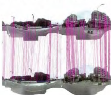
(b)原始全景影像SIFT匹配(去除车体) (b) SIFT match in origin panoramic images
