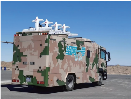
图4 “组网一号”无人机阵列集群快速机动遥感载发车 Fig. 4 “Networking One” drone swarm network rapid remote sensing mobile launch vehicle
