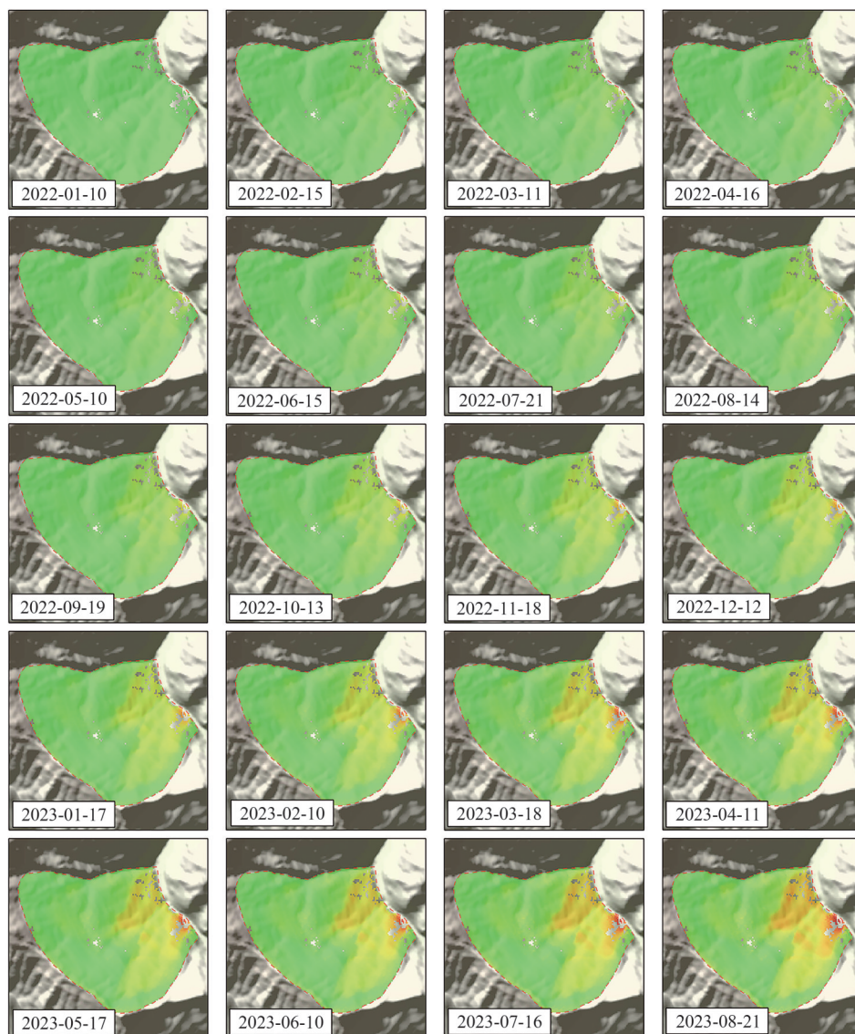
图 11 雄巴滑坡三维形变速率 Fig. 11 Three-dimensional deformation rates of the Xiongba landslide
