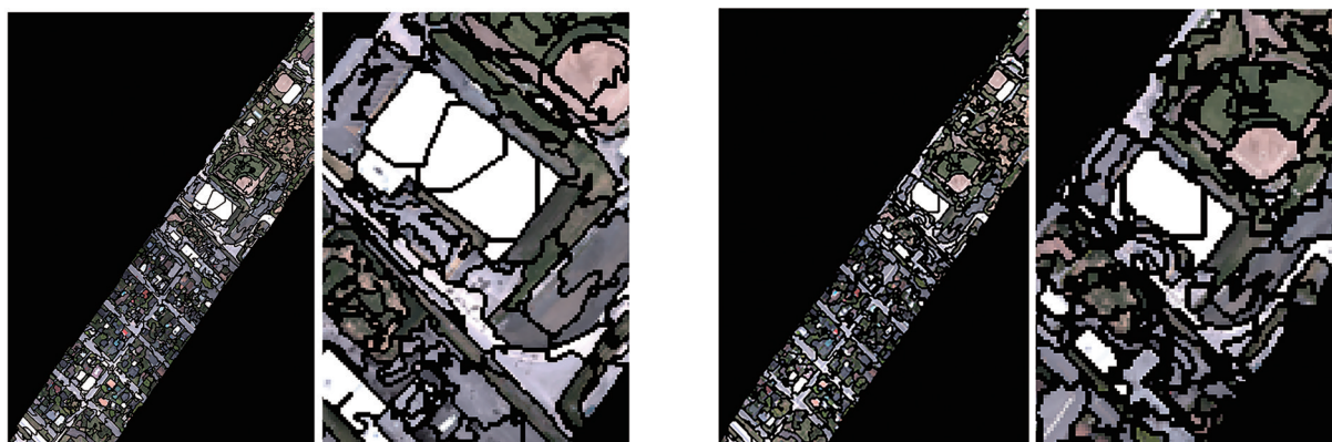
(a) 中分辨率(空间分辨率 1 m)VIS 图像超像素分割结果 (b) 低分辨率(空间分辨率 2 m)VIS 图像超像素分割结果 (a) The result of super-pixel segmentation for mid-resolution VIS image (b) The result of super-pixel segmentation for low-resolution VIS image
