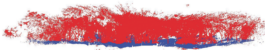
图10 样地A2地面滤波结果(红色为非地面点,蓝色为地面点) Fig. 10 Ground filter result of plot A2 the nonground points and ground points are marked by red and blue colors respectively
